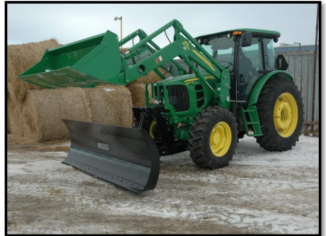
LEON Dozer mounts with NO interference to John Deere factory loader mount. *PLEASE NOTE* Picture only demonstrates mounting capability; tractor or implements not intended for use in this fashion.
